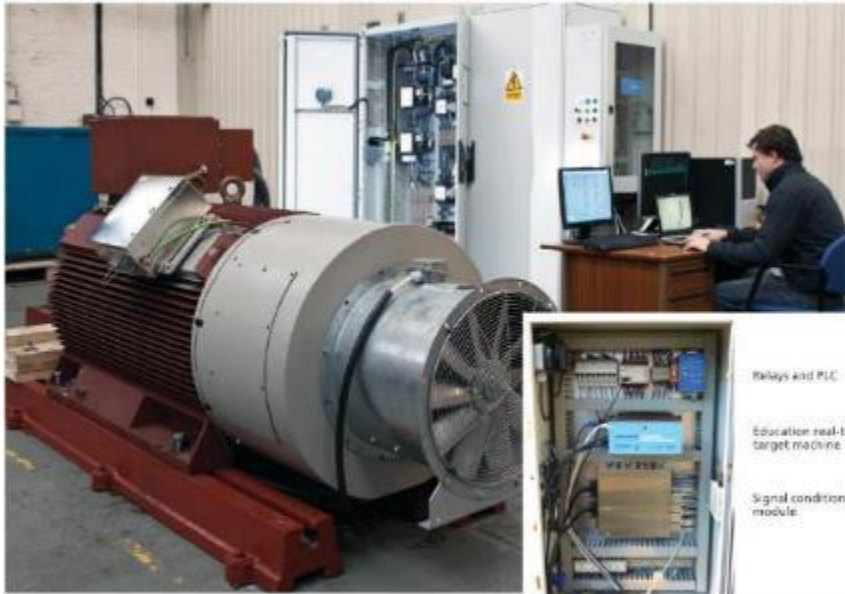
Controlling 250 kW Brushless DFIG using an Education Real-Time Target Machine
